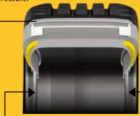
Low heat generating bead filter ensures drivability and durability at zero inflation pressure.
