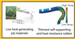
The optimal use of materials and components reduce the size of self-supporting rubber and reduce the stiffness of tire sidewall, improving riding comfort.
