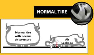
The pressure decreases immediately and the friction produces heat
