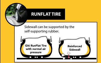
Temporary extended mobility for up to distance of 80km at speed of up to 80km/hr.
